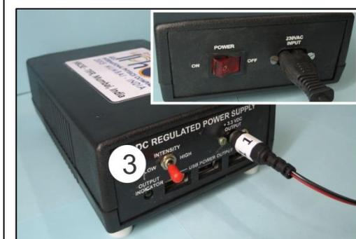
Figure 4: DC regulated power supply
